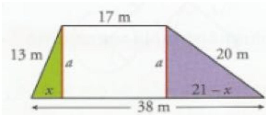
$$\left. \begin{aligned} x^2 + a^2 &= 13^2 \\ (21 - x)^2 + a^2 &= 20^2 \end{aligned} \right\}$$
